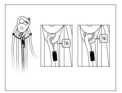
• Check the condition of the sheath over the full length of the rope (cuts, wear, burns, fuzzy areas or signs of chemical products...).
