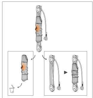
• If necessary, remove the cover and replace it with a JAG SYSTEM replacement cover.
