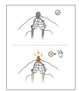
• Check the stitching. Make sure there are no cut, torn, loose, or worn threads.
